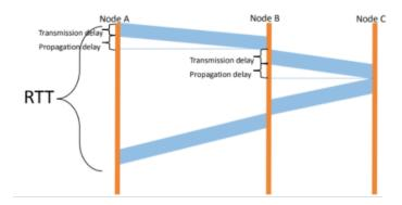
Note the sequence of delays the packet experiences during its route from A to C:
