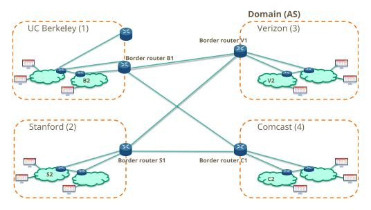
Consider the four ASes in the diagram above. ASes Berkeley, Verizon, Stanford, and Comcast have border routers **B1**, **V1**, **S1**, and **C1** respectively, and internal routers **B2**, **V2**, **S2**, and **C2** respectively.
