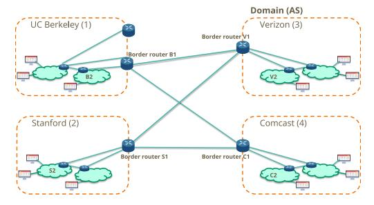
Consider the four ASes in the diagram above. ASes Berkeley, Verizon, Stanford, and Comcast have border routers **B1**, **V1**, **S1**, and **C1** respectively, and internal routers **B2**, **V2**, **S2**, and **C2** respectively.
