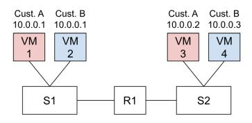
Assume the packets in the underlay network look like the one below. The virtual network header has one field, the ID, which has the name of the customer in it.
