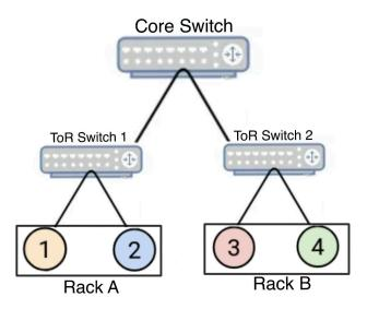
The Clos topology has nodes 1 and 2 in Rack A, nodes 3 and 4 in Rack B, connected via a core switch. Intra-rack links have 1 hop (stretch = 1); inter-rack links have 3 hops (stretch = 3).
