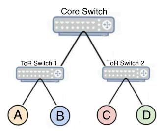
Nodes A and B are in Rack A, nodes C and D are in Rack B, with intra-rack links (stretch = 1) and interrack links (stretch = 3).
