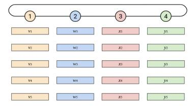
The ring topology connects nodes  $1 \rightarrow 2 \rightarrow 3 \rightarrow 4 \rightarrow 1$  in a closed loop.
